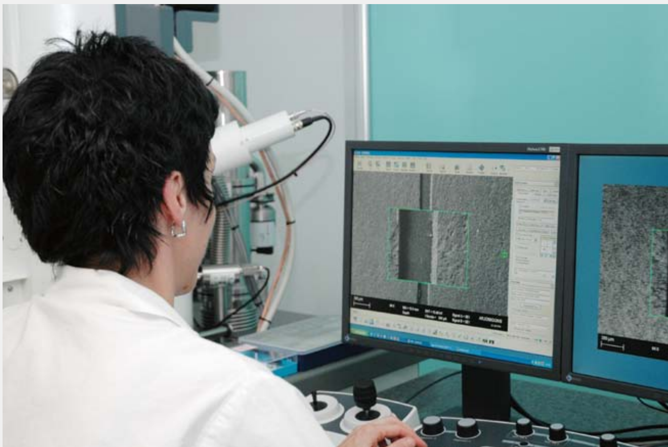
Senior technician Sylvie Faure is using the Scanning Electron Microscope at Apprieu to analyse the surface of a decorative paper.
