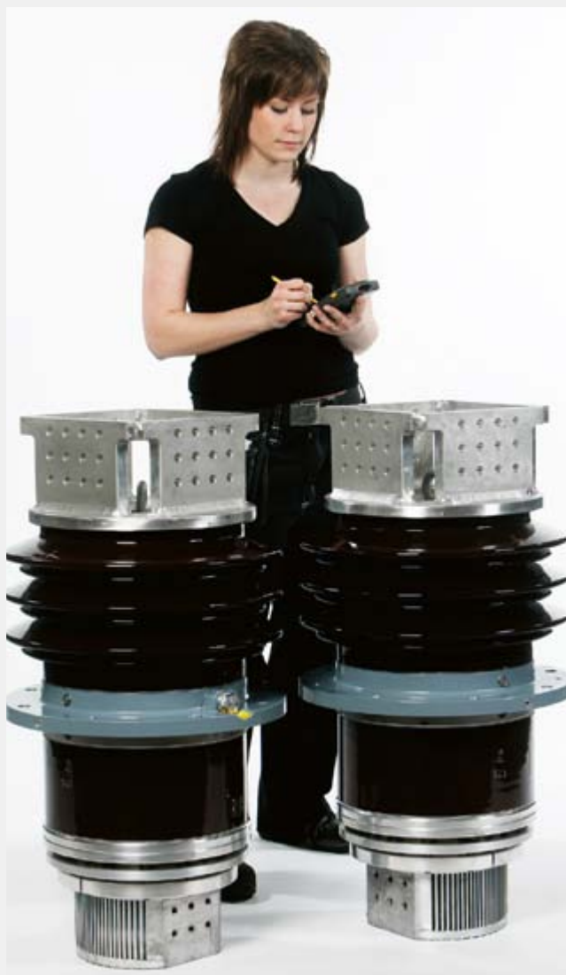
High current bushings type GOH. This product is fitted to the low voltage side on generator step-up transformers. Carries a high current (approx. 25 kA), but the voltage is relatively low, approximately 36 kV.
