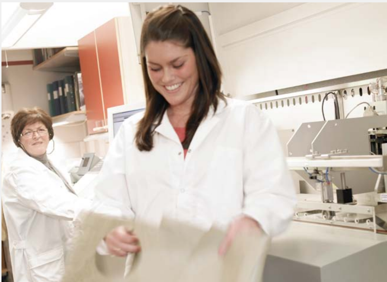
Anna Holmén and Ivana Dusic in the laboratory for Electrotechnical papers in Jönköping performs a CEPI test. CEPI-CTS (Confederation of European Paper. Comparative Testing Service) is performed twice a year to ensure that procedures and equipment give the correct results in the paper test.
